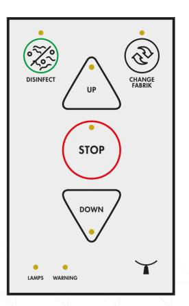
The control panel is simple and functional, also for visually impared people. It houses two controls for raising and lowering the cloth panel, a selection button for disinfecting the fabric, a control for unzipping the cloth panel when it has to be changed, and two warning signals in the event of faulty operation or for changing the UV-C lamp.
